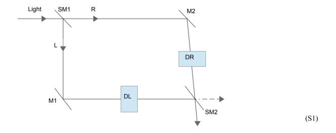
A light ray (starting top left) passes through the depicted test arrangement. The intensity of the light is chosen so low that almost certainly only one single photon is present within the diagrammed area.
